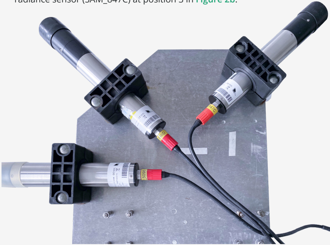
Figure 3. TriOS RAMSES sensors mounted on the steel panel.
