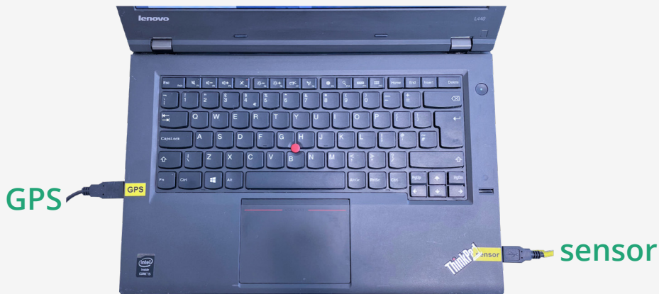
Figure 7. GPS port at the left side and sensor port at the right side of the PC.
