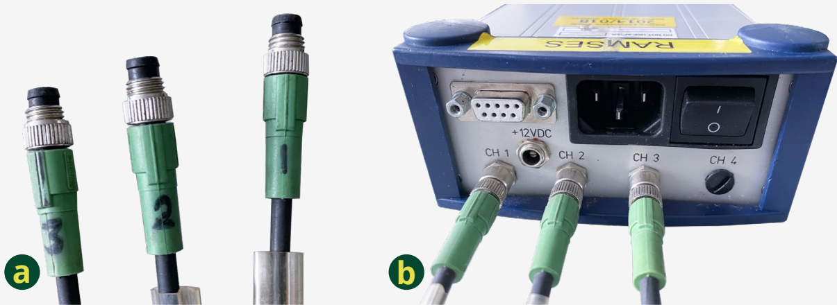
Figure 5. (a) sensor cables with marked number. (b) connected cables to IPS104 interface and power supply unit.
