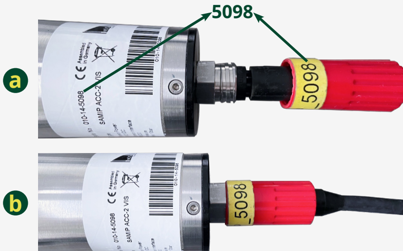
Figure 4. (a) connect the sensor cable. (b) lock the connector
