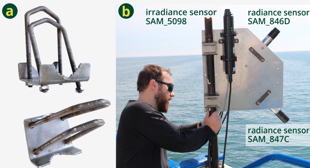
Figure 6. (a) two mast clamps. (b) the position of the steel panel, and the geometry of TriOS sensors.
