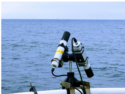
Figure 6.3: Satlantic HyperSAS radiometers mounted on the rotating platform on the bow of RV Plymouth Quest.
