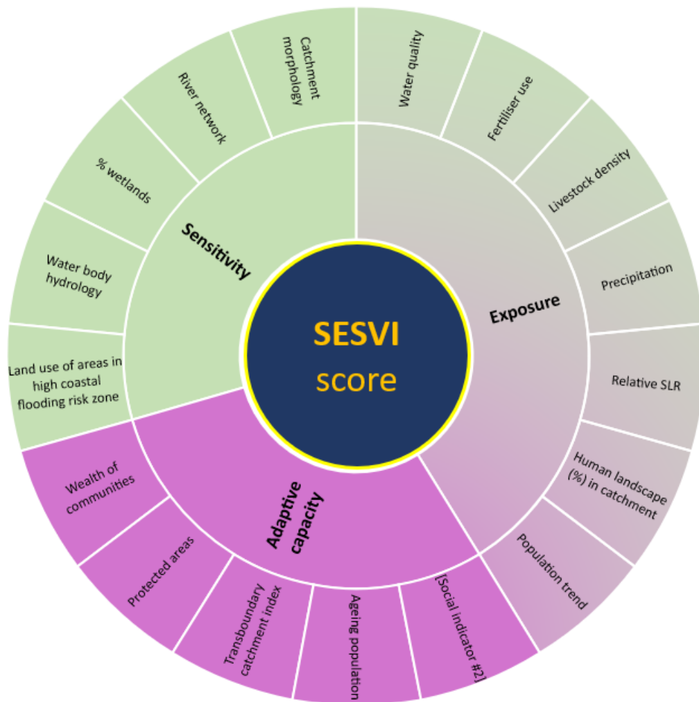
Figure 1. The SESVI wheel summarises in an intuitive visual way the different levels of scoring applied during the application of SESVI. Once applied, a 4-colour traffic-light approach (blue, green, yellow, and red) is used to assign colours to each indicator, component and the SESVI score itself.
