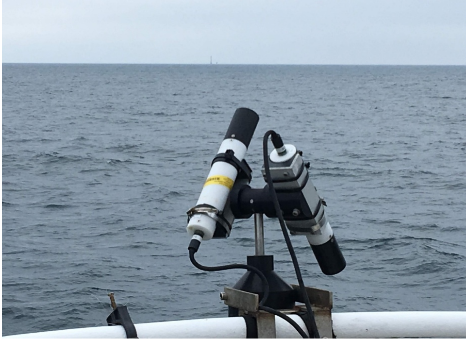
Figure 2. HyperSAS for above-water radiometric measurement (PML)
